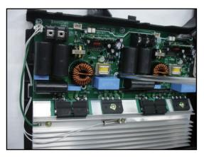
5. Heatsink Sensor wire is hooked. Unhook the wire before taking out the Induction board.
